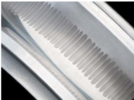
Stray shaft currents discharging through the bearings on rotating equipment can cause fluting on the bearing race, resulting in premature bearing failure.
